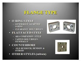
However, O-ring flanges are often attached to equipment that has flat faced pads.
